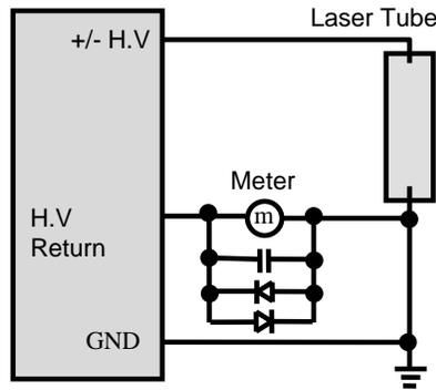
**Output Configuration Wiring (FIG-4)**
