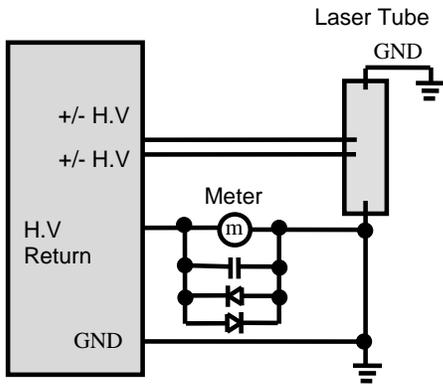
**(4). Single Discharge, One High Voltage, One GND**
